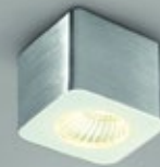
dimmbar, EEK: A E LED 8W, 2800 K, 630 lm, H 55, B 65, L 65
